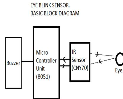
The Sensor Output to the Microcontroller Goes High when the eye is open (Reflecting).
