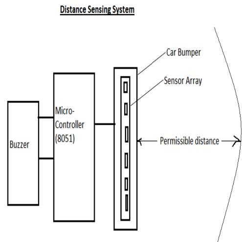
The Buzzer Goes ON when the distance between two vehicles is less than the permissible distnace
