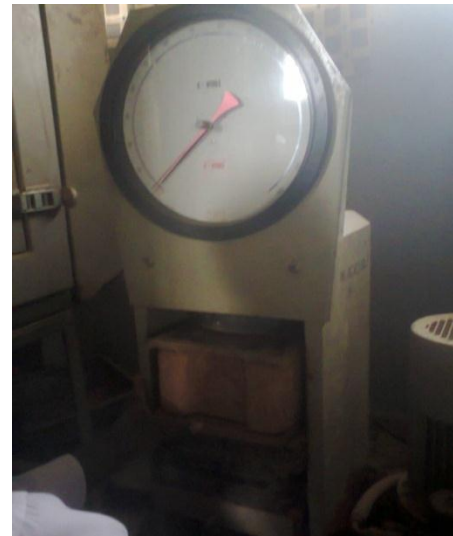
Fig. 4 Crushing of CSEB on Compressive Strength Testing Machine
