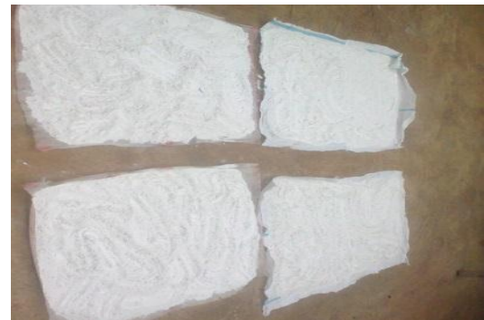
Fig. 3 Air Drying of Wet Milled Waste Glass under the Sun
