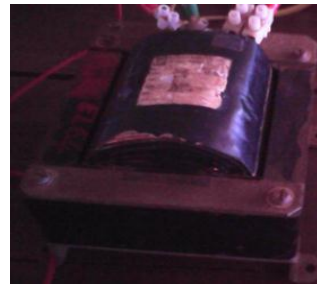
Fig. 4. Photograph of the Single Phase Transformer Understudy
