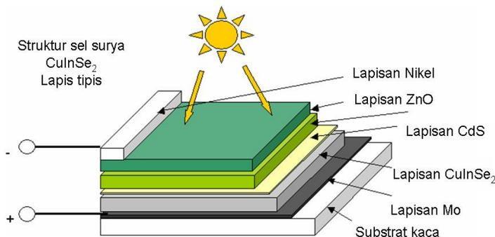
Struktur sel surya = Structure of solar cell
