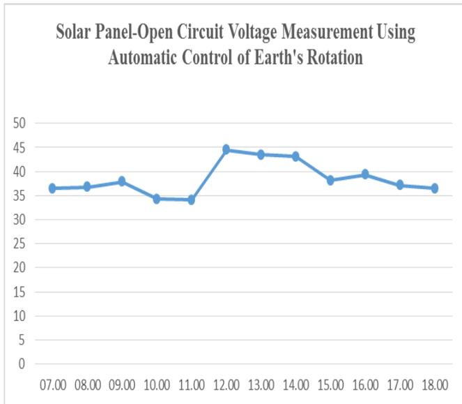
**Figure 4.4.** Chart of Open Circuit Voltage Measurement
