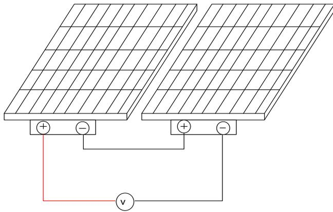
**Figure 10.** Diagram of Solar Panel-Open Circuit Voltage Test
