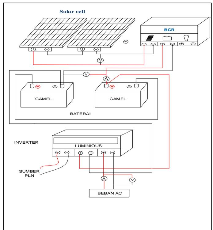
Figure 15. Circuit of Testing with AC Load
