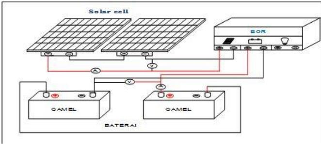
Figure 15. Circuit of Battery Charging and Zero Load
