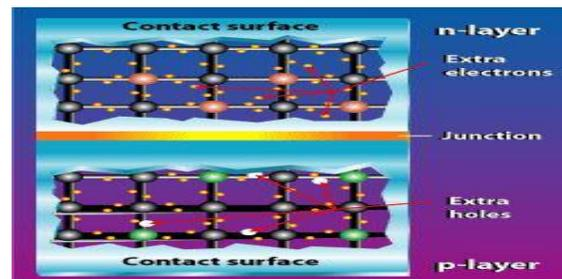
**Image 2:** Junction between p-type and n-type semiconductors
