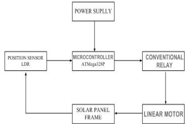
**Figure 9.** Solar Tracker Control System
