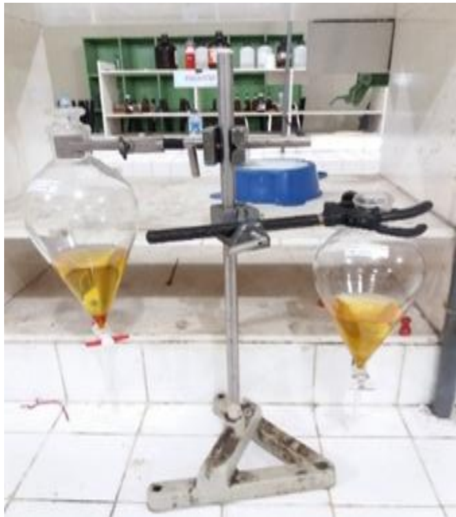
Figure 2. Two Phases Layer in Transesterification Process.
