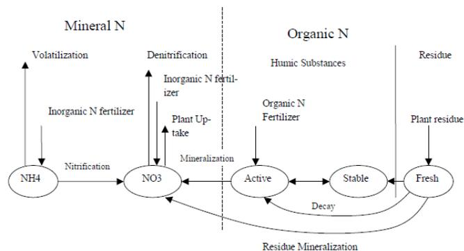
**Fig. 1** SWAT Soil Nitrogen and Processes that Move Nitrogen in And Out of Pools (Neitsch, 2002).
