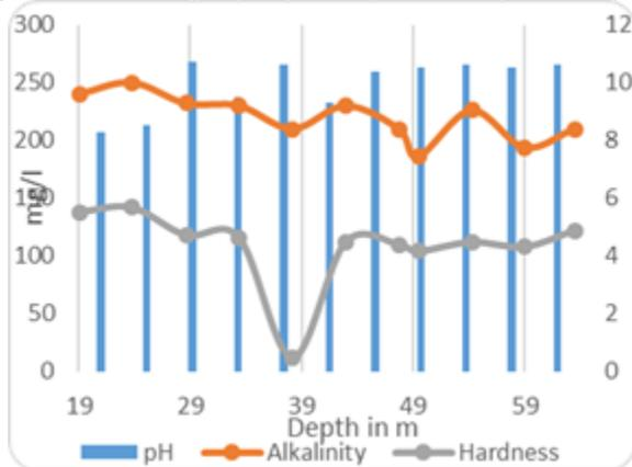
**Fig. 3.3** Variation of pH, Alkalinity and Hardness along the depth
