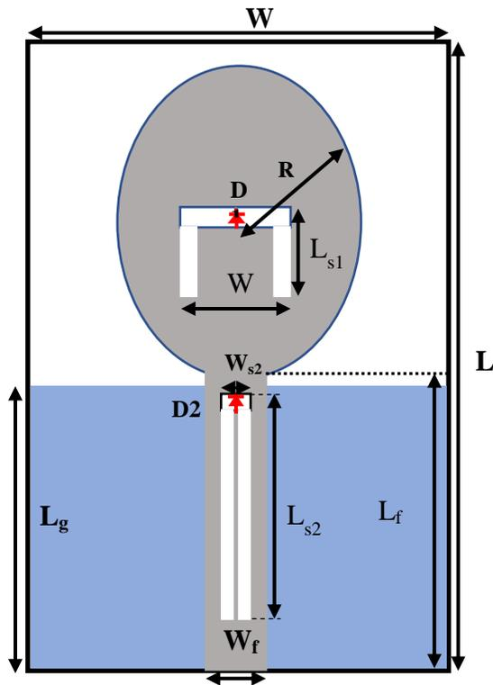
Fig. 1. Layout of proposed circular monopole antenna with two reversed U-shaped slots.
