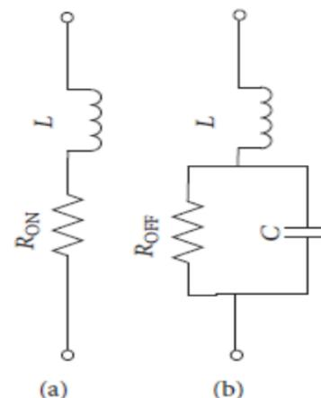
Fig. 2. Simplified model of PIN diode (a) Forward biasing and (b) Reverse biasing.
