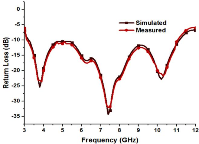
**Fig. 3.** Comparison between simulated and experimental return loss when both diodes are ON.
