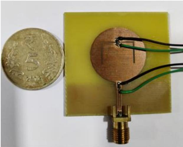
**Fig. 10.** Photograph of the prototyped antenna.
