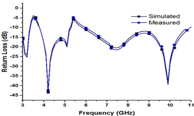
**Fig. 4.** Comparison between simulated and experimental return loss when both diodes are OFF.
