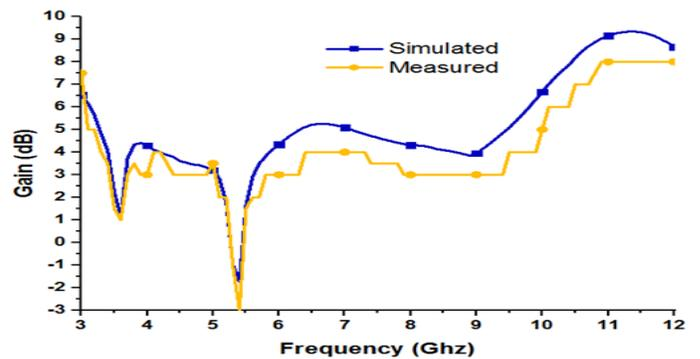
**Fig. 7.** Comparison between simulated and experimental Gain of the antenna when both diodes are OFF
