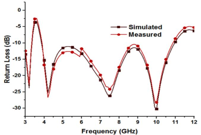
**Fig. 5.** Comparison between simulated and experimental return loss when D1 is OFF and D2 is ON.
