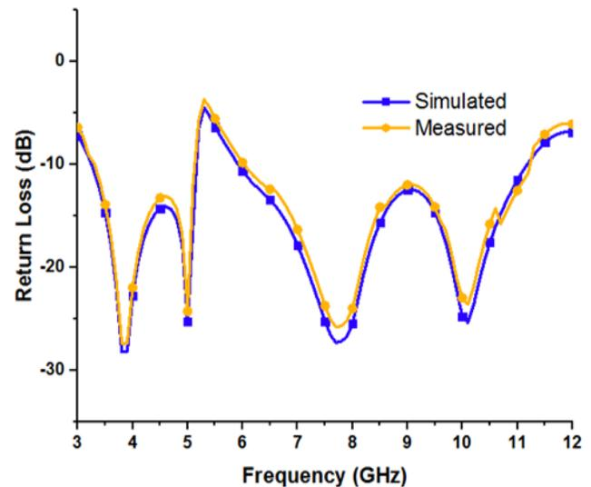
**Fig. 6.** Comparison between simulated and experimental return loss when D1 is ON and D2 is OFF.
