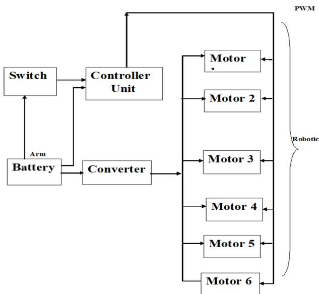
Fig. 1. Block diagram of the feeding device
