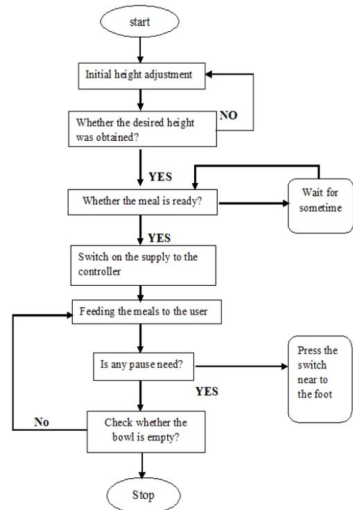
Fig. 2. Flowchart of the Assistive Feeding Device.
