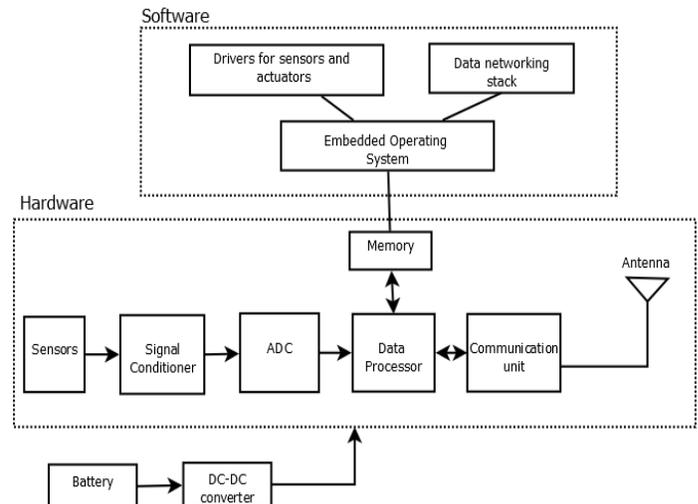
Figure 1: Architecture of Wireless Sensor Node
