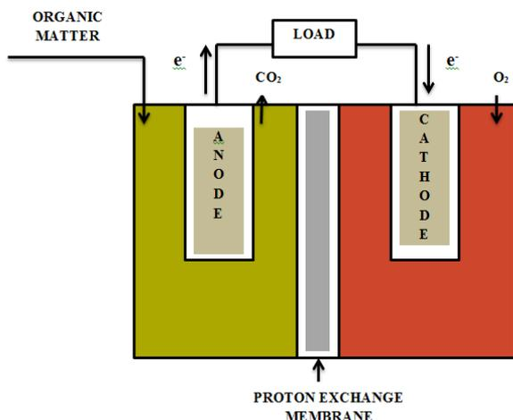
**Fig. 3** Schematic of Dual Chamber MFC
