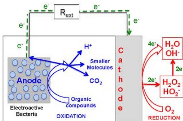
Fig. 1 Schematic of MFC [26]
