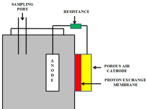
Fig. 2 Schematic of Single Chamber MFC
