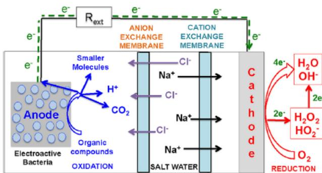
Fig. 4 Microbial Desalination Cell [26]
