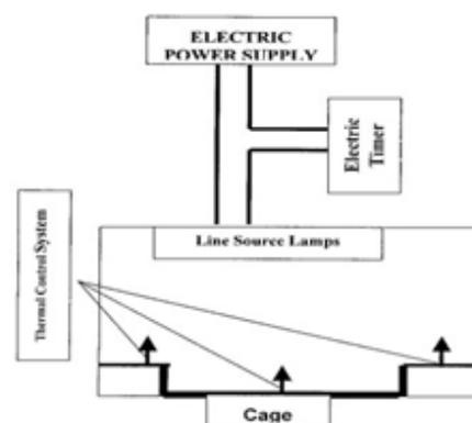
Fig. 1: Arrangement for application of electromagnetic field
