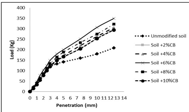
FIG. 3. LOAD PENETRATION CURVE FOR VARIOUS PROPORTIONS MM
