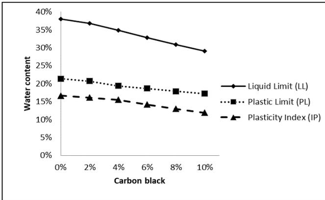
FIG. 1. EFFECT OF CARBON BLACK ON ATTERBERG'S LIMIT
