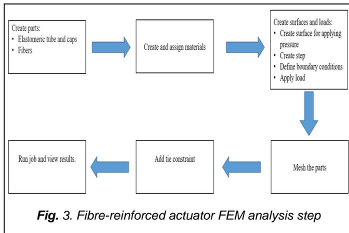
Fig. 3. Fibre-reinforced actuator FEM analysis step
