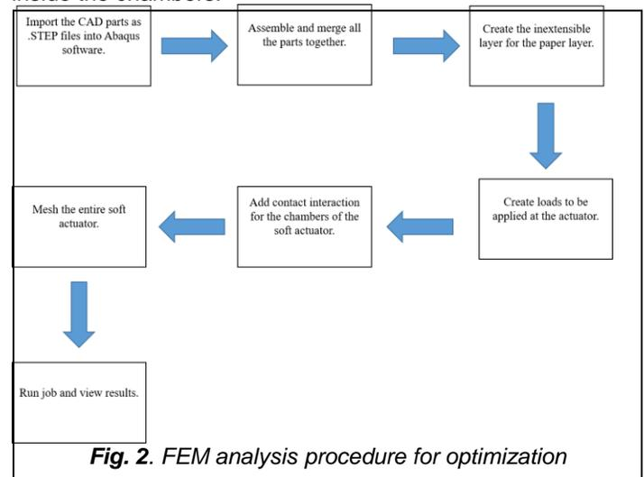
**Fig. 2. FEM analysis procedure for optimization**
