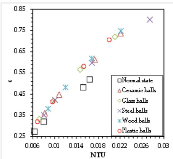
Fig. 12 Relation between  $\epsilon$  and NTU for counter flow when  $V_h$  is 4 LPM
