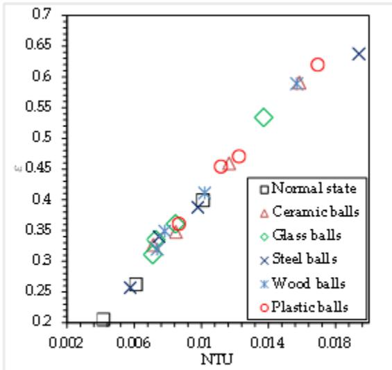
Fig. 7 Relation between  $\epsilon$  and NTU for parallel flow when  $V_h$  is 3 LPM
