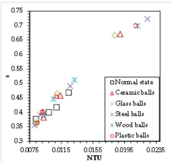
Fig. 11 Relation between  $\epsilon$  and NTU for counter flow when  $V_h$  is 3 LPM
