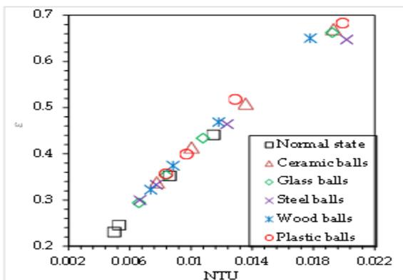
Fig. 8 Relation between  $\epsilon$  and NTU for parallel flow when  $V_h$  is 4 LPM.
