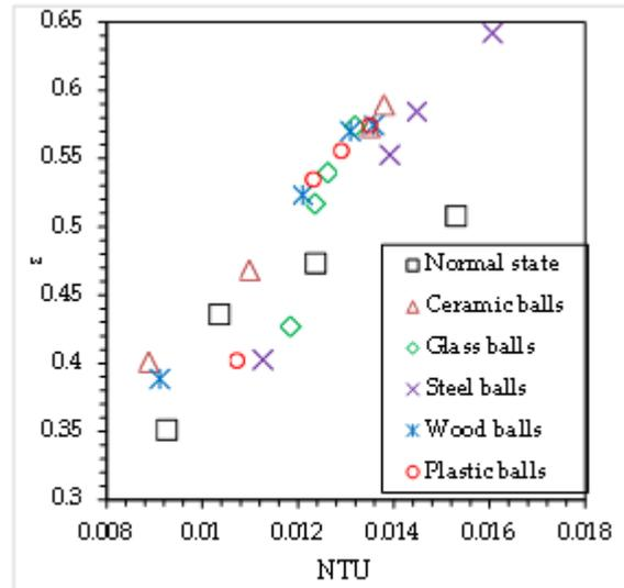
Fig. 9 Relation between  $\epsilon$  and NTU for counter flow when  $V_h$  is 1 LPM.
