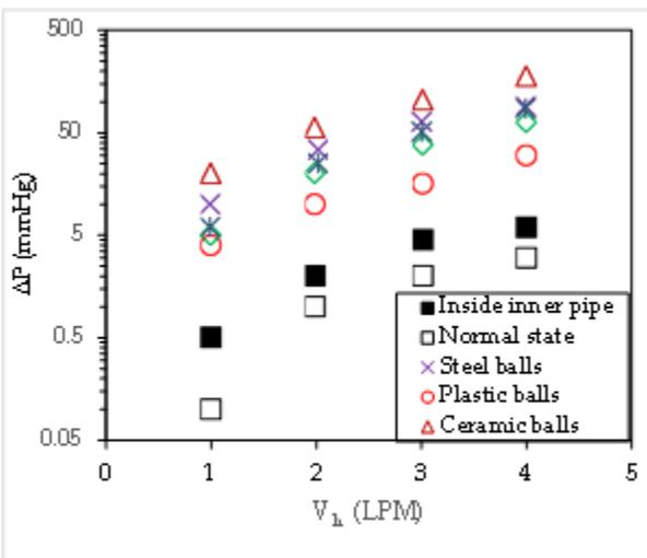
Fig. 13 Variation of pressure drop relative to the fluid flowrate
