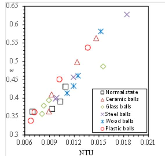
Fig. 10 Relation between  $\epsilon$  and NTU for counter flow when  $V_h$  is 2 LPM
