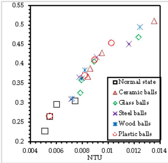
Fig. 6 Relation between  $\epsilon$  and NTU for parallel flow when  $V_h$  is 2 LPM
