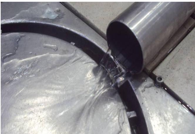
**Figure 8: Bottle rinse water being channeled to the drain**
