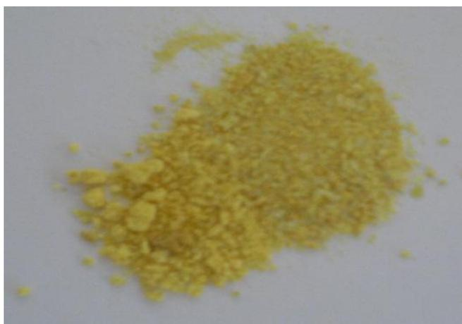
**Fig. 3 Product obtained after decomposition of fully cured samples of Araldite DLS 772 / 4 4' DDS with an amine / epoxy ratio of 0.8 after decomposition at 120°C for a total of 75 minutes in Microwave Reaction System.**
