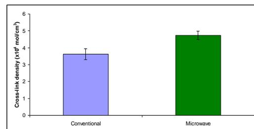
**Fig 8 Plot of Bar chart of cross-link density values of conventional and microwave cured samples of Araldite DLS 772 / 4 4' DDS epoxy system with an amine / epoxy system of 0.8**
