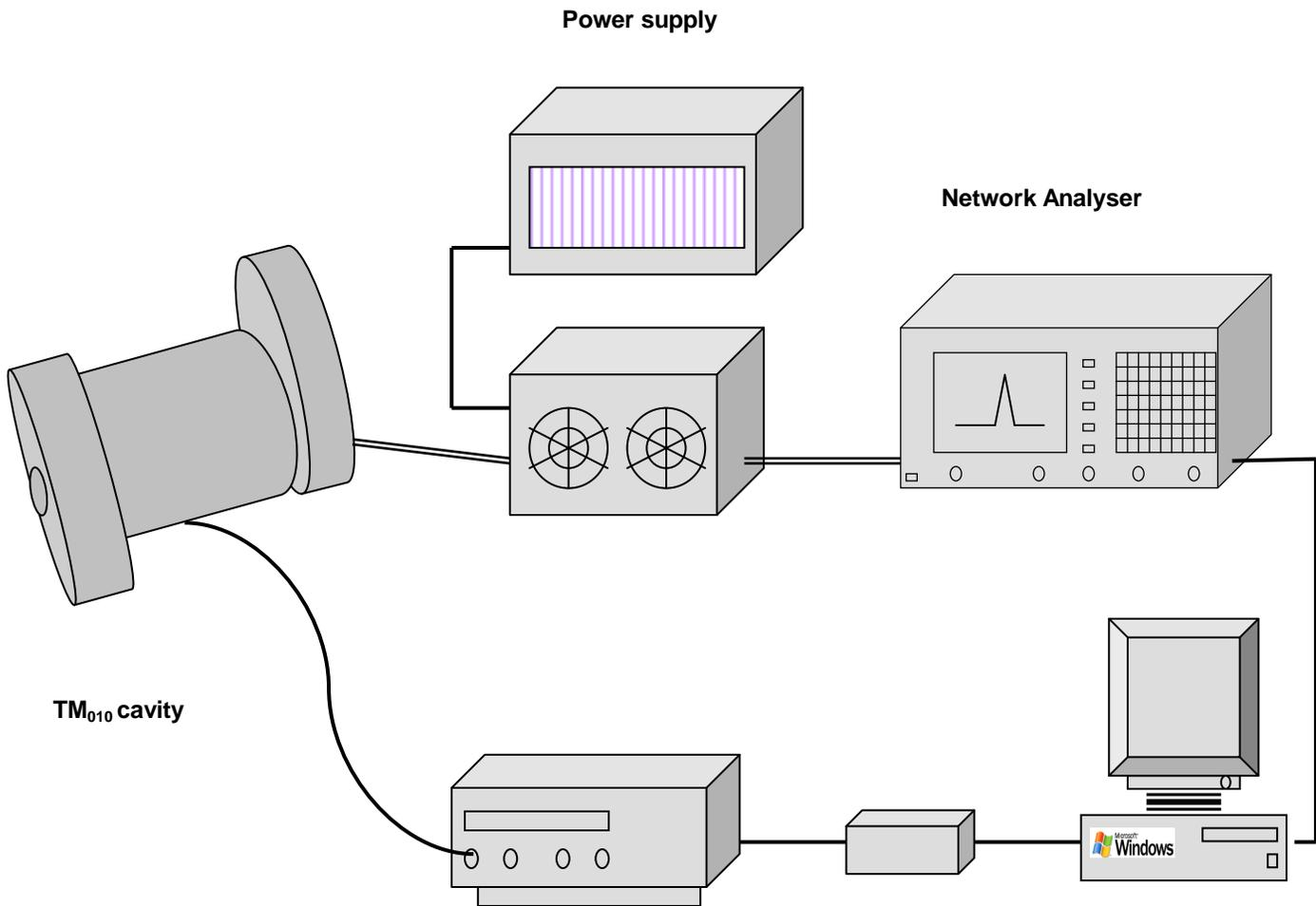
**Fig. 2 A schematic diagram of a microwave heating system using a single mode cavity operated in TM<sub>010</sub> mode [5]**
