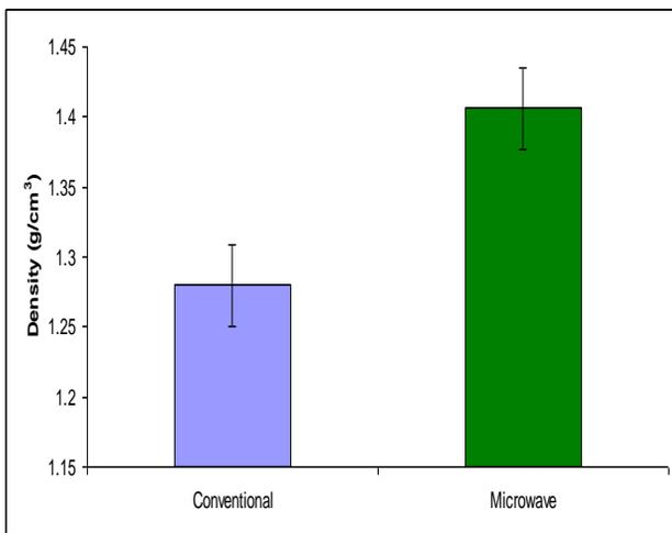
**Fig. 4** Plot of Average Density for conventionally and microwave cured samples of Araldite DLS 772 / 4 4' DDS epoxy system with an amine / epoxy ratio of 0.8
