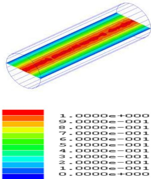
**Fig. 1 Simulated electromagnetic field patterns at 2.45GHz for TM<sub>010</sub> mode microwave cavity with the presence of sample generated using Ansoft HFSS v8.5 simulation software. The colour scale shows the relative field strength generated inside the cavity [5]**
