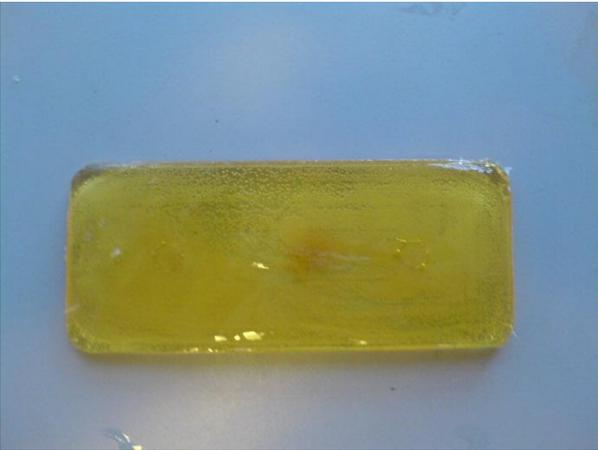
**Fig. 3** Fully cured sample of Araldite LY 5052 / 4 4' DDS epoxy system with an amine / epoxy ratio of 0.8 with microwave heating at 180°C for 240 minutes.
