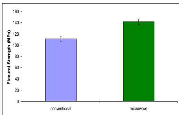
Fig.11 Bar chat of Average flexural strength values of conventional and microwave cured samples of Araldite.
