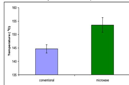
**Fig 7 Bar chart of Average T<sub>g</sub> values of conventional and microwave cured samples of Araldite DLS 772 / 4 4' DDS epoxy system with an amine / epoxy ratio of 0.8.**
