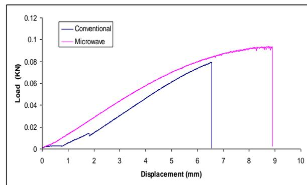
**Fig. 10 Load vs Displacement plot for conventional and microwave cured samples of Araldite DLS 772 / 4 4' DDS epoxy system with an amine / epoxy ratio of 0.8.**
