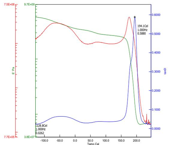
**Fig. 5** Dependence of storage modulus ( $G'$ ), Loss modulus ( $G''$ ) and  $\tan \delta$  with temperature for a fully cured sample of Araldite DLS 772 / 4 4' DDS epoxy system with an amine / epoxy ratio of 0.8 prepared using conventional heating at 180°C for 240 mins.
