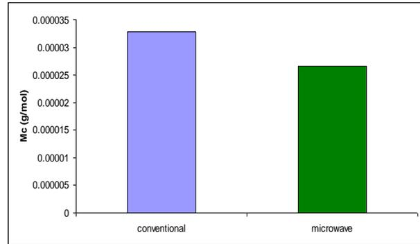
**Fig. 9 Plot of average molecular weight between cross-links ( $M_c$ ) of conventional and microwave cured samples of Araldite DLS 772 / 4 4' DDS epoxy system with an amine / epoxy ratio of 0.8 using Nielsen's equation.**
