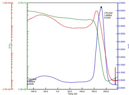
**Fig. 6 Dependence of storage modulus (G'), Loss modulus (G'') and tan δ with temperature for a fully cured sample of Araldite DLS 772 / 4 4' DDS epoxy system with an amine / epoxy ratio of 0.8 prepared using microwave heating at 180 °C for 240 mins.**
