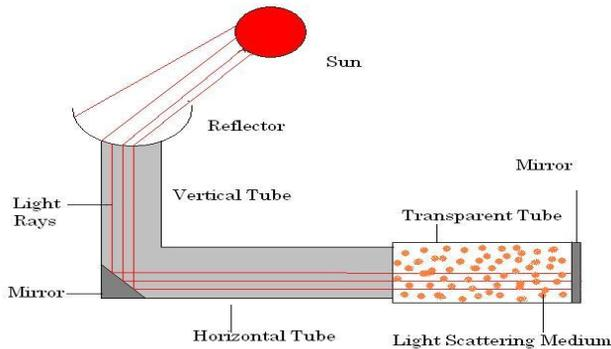
**Fig 1:-** The schematic layout of the conventional solar tube system.
