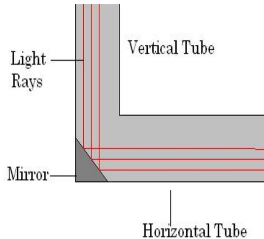
Fig 6:- The view of the horizontal, vertical tube with a mirror arrangement
