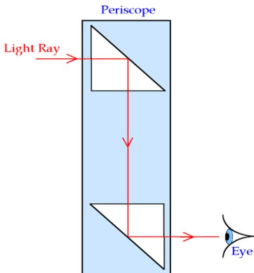
Fig 5:- The schematic view of periscope using two prisms
