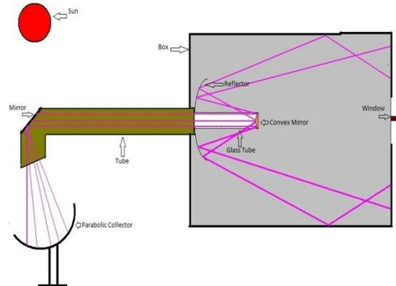
**Fig 2:-** Modified Solar Tube system
