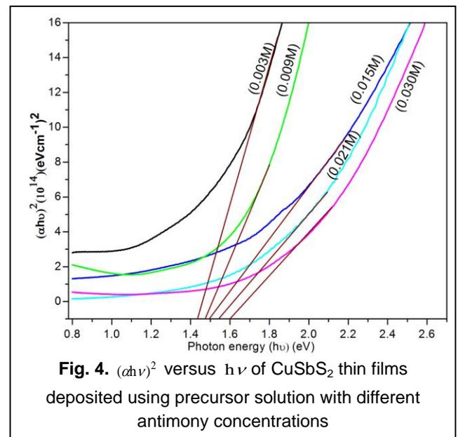
**Fig. 4.**  $(\alpha h\nu)^2$  versus  $h\nu$  of CuSbS<sub>2</sub> thin films deposited using precursor solution with different antimony concentrations
