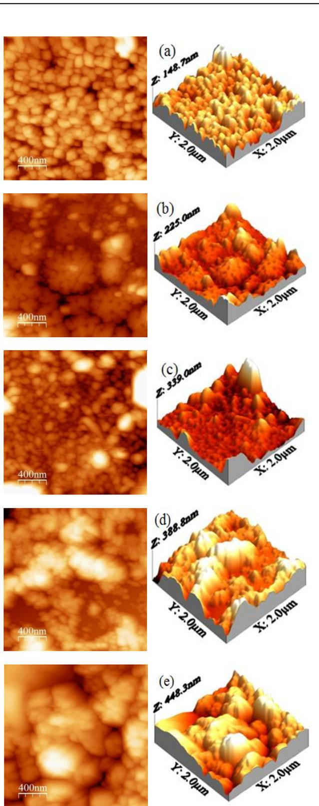
**Fig. 3.** 2D and 3D AFM micrographs of CuSbS<sub>2</sub> thin films deposited using precursor solution with different antimony concentrations: (a) 0.003M, (b) 0.009M, (c) 0.015M, (d) 0.021M, (e) 0.03M
