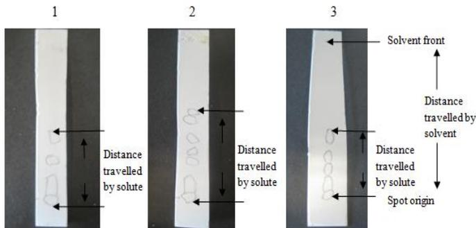
**Fig.3.** Thin layer chromatography when view under ultraviolet light chamber after immersed with samples solvent. 1: P550A1a, 2: P550A1b, 3: P550A1c.
