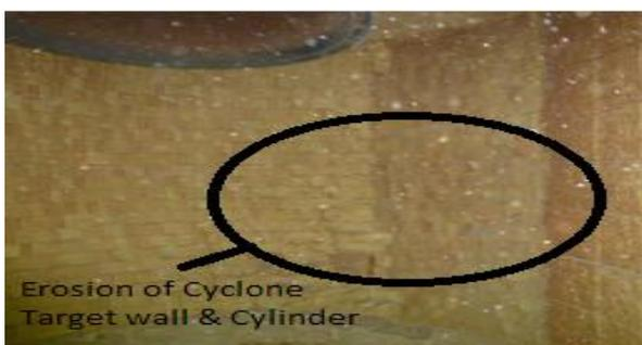
**Figure 4.** Photograph of Erosion in Cyclone Target Area
