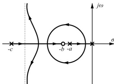
Fig 2-b. Two distinct break points between zero  $s = -b$  and adjacent pole  $s = -c$ .
