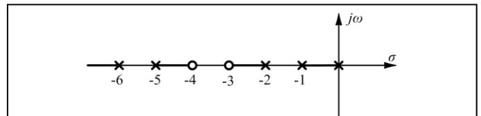
Fig 3-a. The root locus of (4) on the real axis for  $k > 0$
