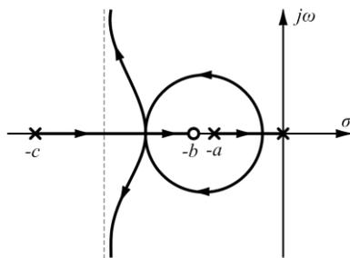
Fig 2-c. Double break point the between zero  $s = -b$  and adjacent pole  $s = -c$ .
