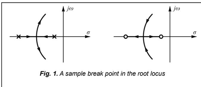
Fig. 1. A sample break point in the root locus
