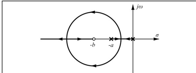
Fig 2-a. Existence of break point between two adjacent poles ( $s = 0, s = -a$ ) and between two adjacent zeroes ( $s = -b, s = -\infty$ )
