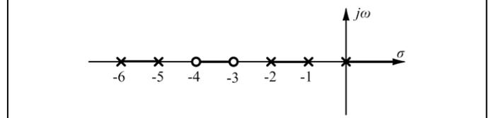
Fig 3-b. The root locus of (4) on the real axis for  $k < 0$
