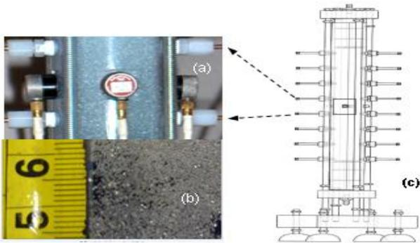
**Fig.1.** (a) Measurement configuration of (dry) granular analogue, and (b) material size (0.5mm spherical ceramic spheres). (c) Granular analogue (45cm x 5cm) confined in the instrumented flow-cell with ultrasonic P- and S-wave source-receiver sensor pairs attached midspan.
