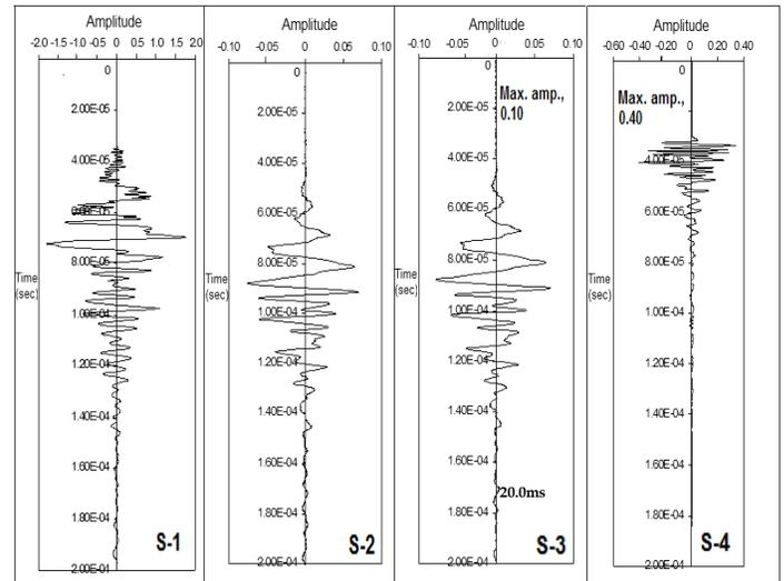
**Fig.4.** Acquired, ultrasonic S-waves, S 1-3 dry and - 4 brine saturated.
