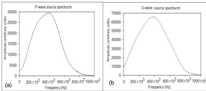
**Fig.5.(a) P-wave, and (b) S-wave transmitted spectral characteristics.**
