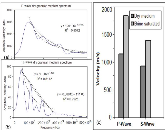
**Fig.6. (a) P-wave, and (b) S-wave received (measurement) spectral characteristics. (c) Velocity estimates corresponding to Fig.3 and Fig.4.**
