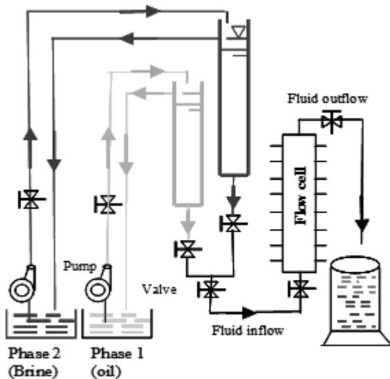
**Fig.2.** Schematic of flow control system facilitated immiscible fluid-displacement process through the (saturated) granular analogue.
