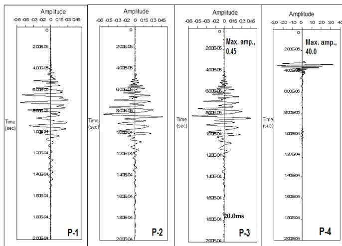
**Fig.3.** Acquired, ultrasonic P-waves, P 1-3 dry and – 4 brine saturated.
