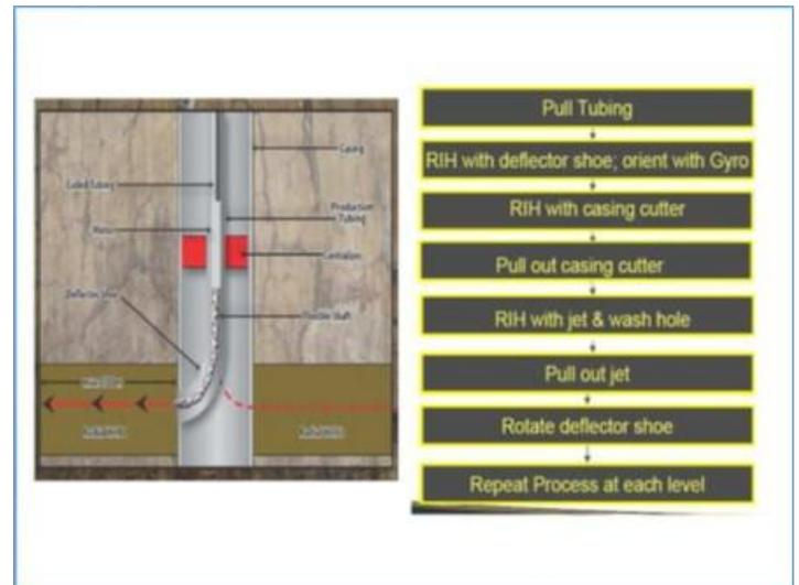
**Fig. 2:** RJD procedure (Courtesy of RadJet).
