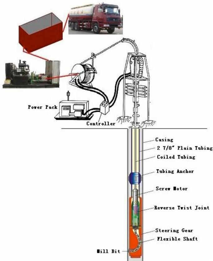
Fig. 8: Equipment connection diagram.
