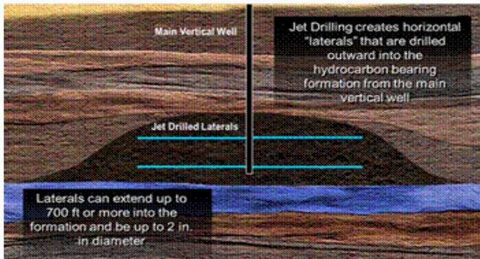
**Fig. 1:** Radial jet drilling (Courtesy of Buckman Jet Drilling)
