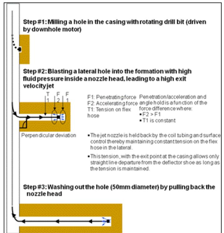
**Fig. 3:** RJD procedure (Courtesy of RadJet).
