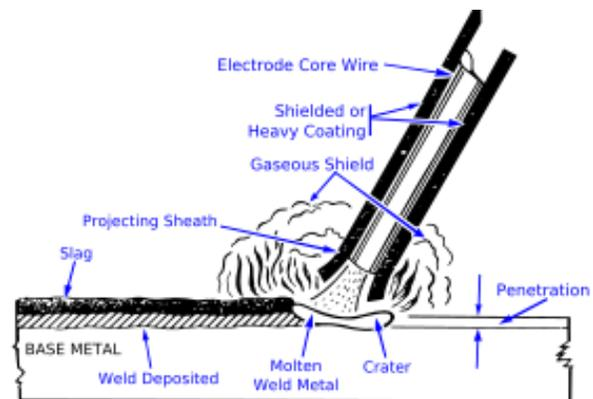
Figure 1. Shielded Metal Arc Welding [4]
