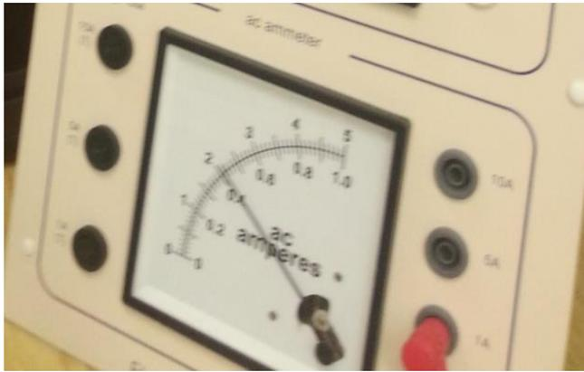
Fig. 5. AC ammeter reading 0.4A
