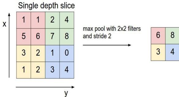
Figure 6: Two cross two max pooling
