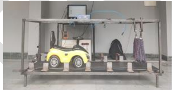
Fig.3 Snapshot of Automatic Vehicle Washing System
