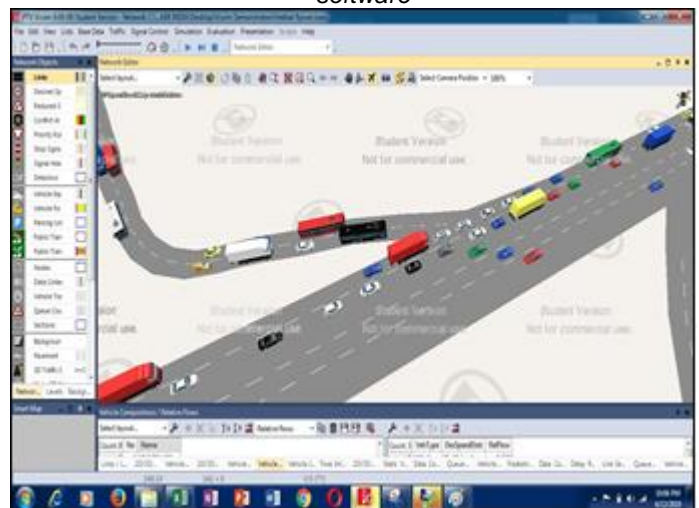
Fig-5. Queue being formed observed at junction in VISSIM software
