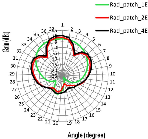
**Fig 9 :** Elevation pattern gain for 1,2 and 4-element microstrip patch array
