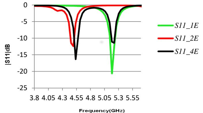
Fig 8 : RL for 1,2 and 4-element microstrip patch array
