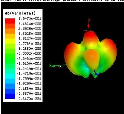
**Fig 10 :** 3D pattern view of the array of 4-element
