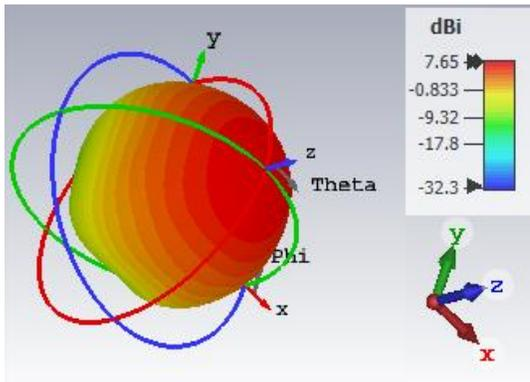
**Fig. 13.** E field simulation results of this human uterus phantom model without tumour
