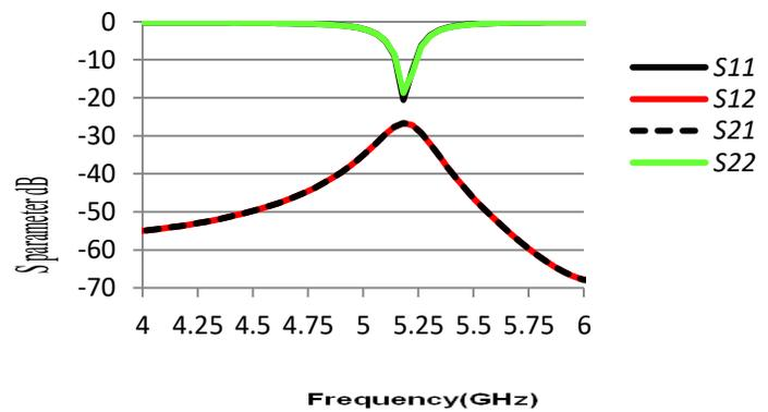
Fig. 7. RL for double patch element with  $\lambda$  distance
