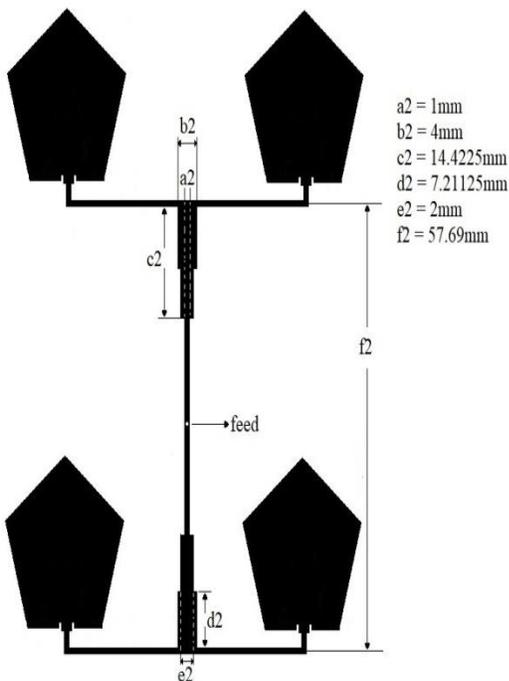
Fig. 6. Geometry of a four elements microstrip patch antenna array
