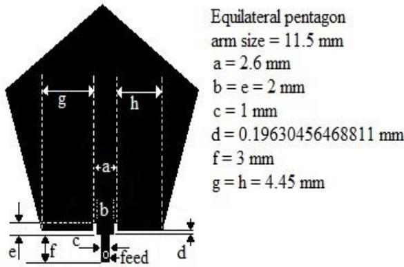
Fig 4. Geometry of a single element microstrip patch antenna
