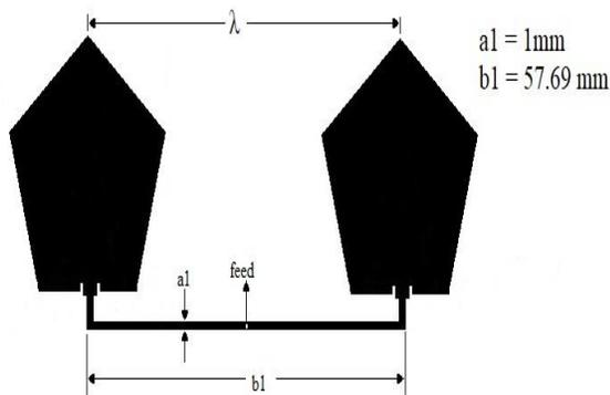
Fig 5. Geometry of a double elements microstrip patch antenna array
