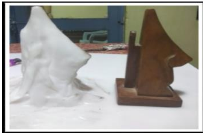
Fig 9: Pattern and Formed Product of a Wooden Handcraft
