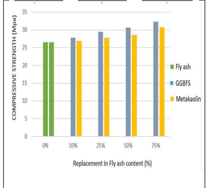
**Fig. 2.** Graphical Representation of Compressive strength at 7 days Curing Period. The result indicates that the increase in the replacement of mineral admixtures in fly ash content leads to improvement in the early age strength.
