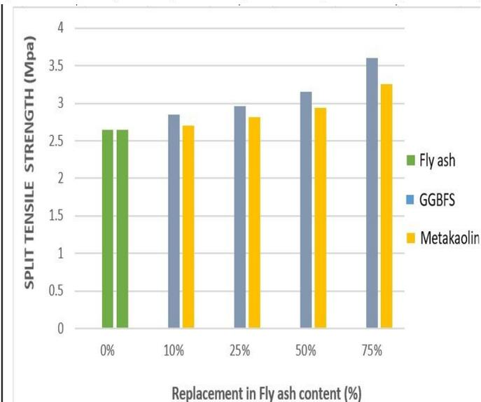
**Fig. 3.** Graphical Representation of Split Tensile strength at 7 days Curing Period. The result indicates that as same as compressive strength. An increase in the replacement of mineral admixtures in fly ash content leads to improvement in the early age strength.
