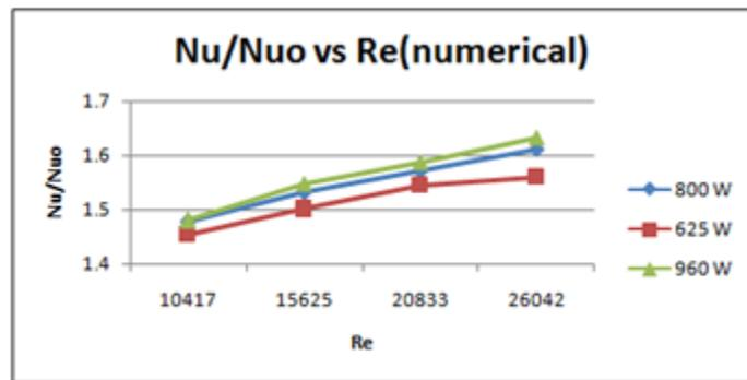
**Fig. 12** Effect of Re on heat transfer enhancement for different heater inputs for truncated stepped grooved rib
