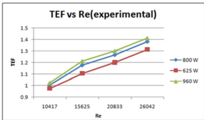
**Fig. 10** Effect of Re on Thermal Enhancement factor for truncated stepped grooved rib for all heater inputs
