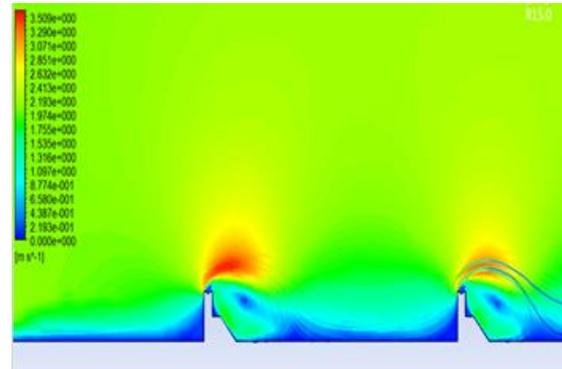
Fig. 4 Velocity profile of Truncated stepped grooved shoe shape rib
