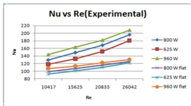
**Fig. 7.** Effect of Re on Nu for different heater inputs for truncated stepped grooved rib and Flat plate
