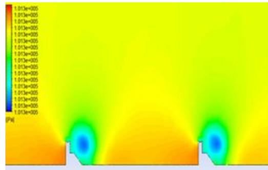
Fig. 5 Pressure profile of Truncated stepped grooved shoe shape rib
