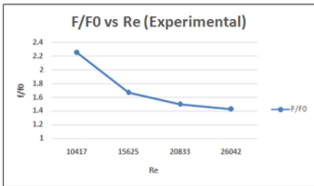
**Fig. 9** Effect of Re on friction factor ratio for truncated stepped grooved rib
