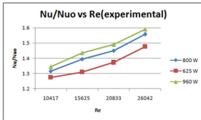
**Fig. 8** Effect of Re on heat transfer enhancement for different heater inputs for truncated stepped grooved rib
