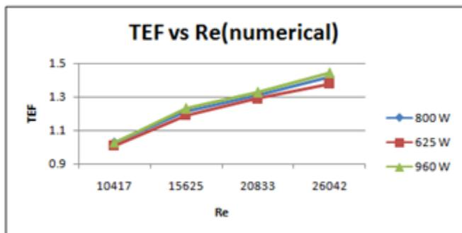
**Fig. 13** Effect of Re on Thermal Enhancement factor for truncated stepped grooved rib for all heater inputs
