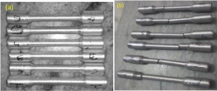
Fig. 6. Image of the specimens (a) before tensile test (b) after tensile test
