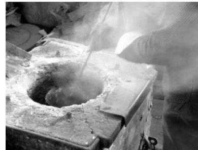
**Fig. 2.** Image of the Stir casting process.
