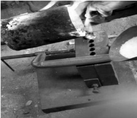
*Fig. 4. Melting and streaming process for tensile test.*
