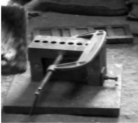
*Fig. 3. Dies for tensile testing specimens.*
