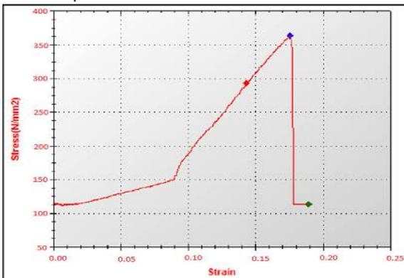
**Fig. 10.** Graph of Stress Vs Strain at composition (97%Al, 2%Mo, 1%CSA)
