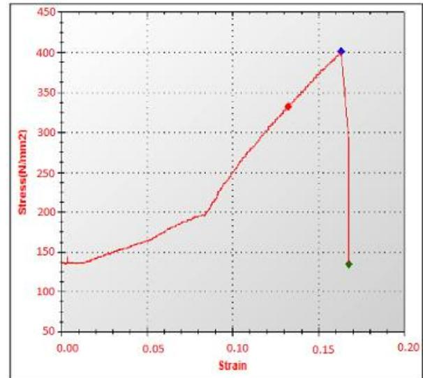
**Fig. 11.** Graph of Stress Vs Strain at composition (97%Al, 4%Mo, 1%CSA)
