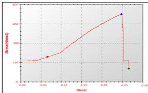
Fig. 7. Graph of Stress Vs Strain at composition (97%Al, 1%Mo, 2%CSA)
