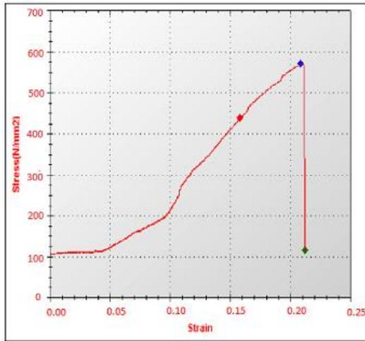
**Fig. 9.** Graph of Stress Vs Strain at composition (93%Al, 1%Mo, 6%CSA)
