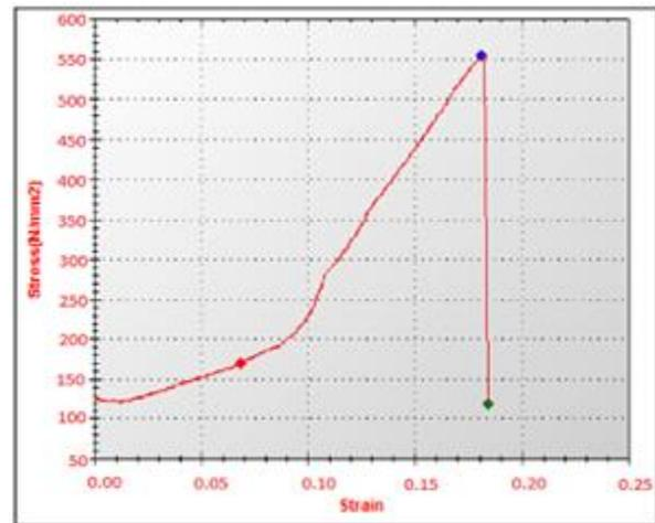
**Fig. 12.** Graph of Stress Vs Strain at composition (97%Al, 6%Mo, 1%CSA)
