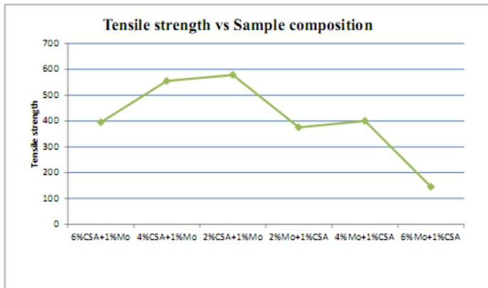
**Fig. 14.** Graph between sample composition and tensile strength.
