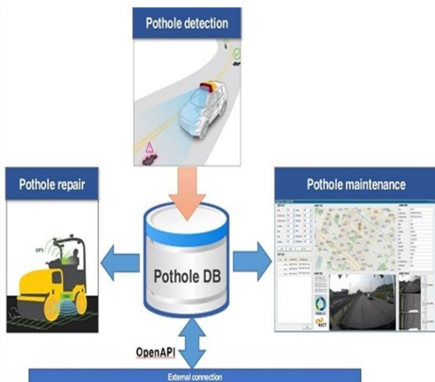
Fig 1: Overall Block diagram of Pothole detection system
