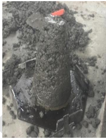
(a) Slump test
