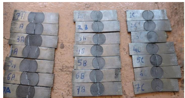
Fig 2.4 Samples after Tensile testing
