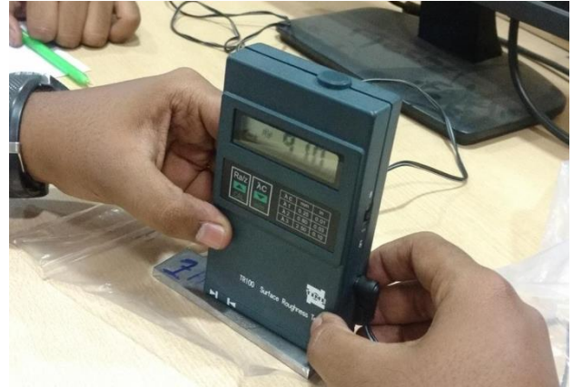
Fig 2.3 Surface roughness testing
