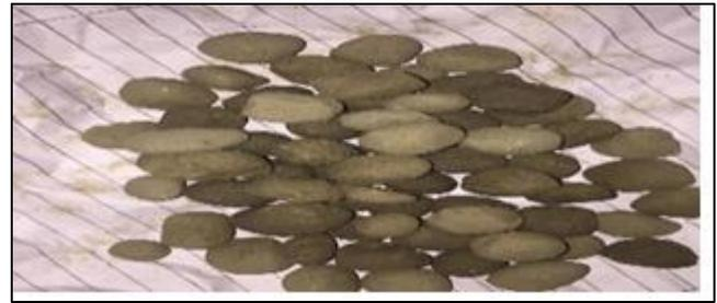
**Fig 5:** Oven dried loaded expansive clay particles with bacteria cell (healing Agent).
