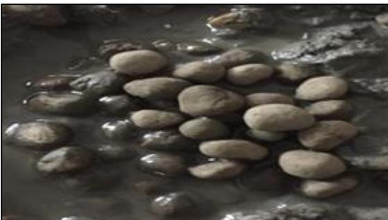
**Fig 9:** mixing oven dried loaded expansive clay particles with concrete.
