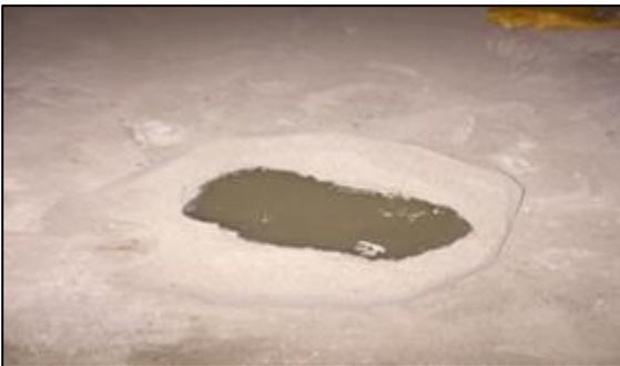
**Fig 7:** Pumice immobilized bacterial cell solution in sand and cement mixture.
