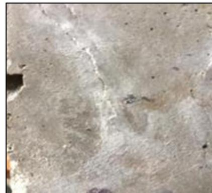
**Fig 31:** Stiffen sand capsule concrete with crack width of 0.018 mm partially sealed by  $\text{CaCO}_3$  precipitate from the crack tip.
