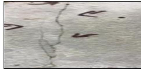
**Fig 29:** Pumice immobilized bacterial concrete with crack width of 0.015 mm completely sealed by  $\text{CaCO}_3$  precipitate from the crack tip.
