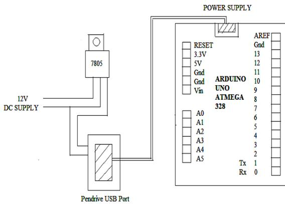
**Fig. 8.** Voltage Regulator 7805 with Arduino
