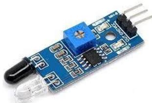
**Fig. 10.** Infrared sensor module
