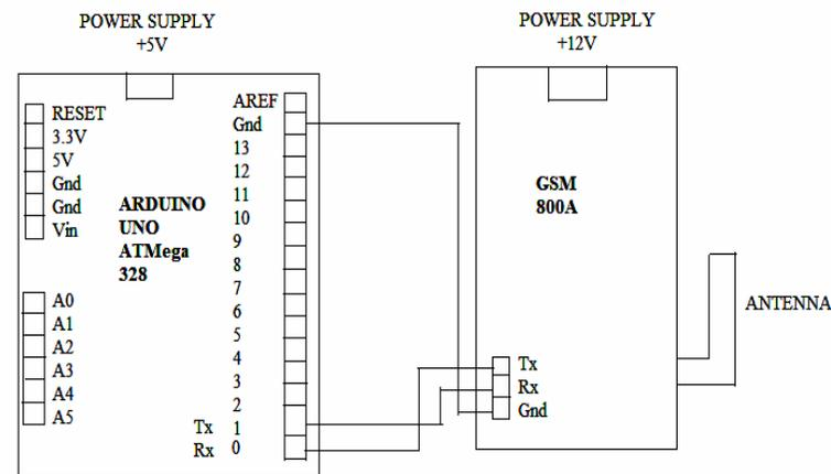
Fig. 6. Arduino Interfacing with GSM
