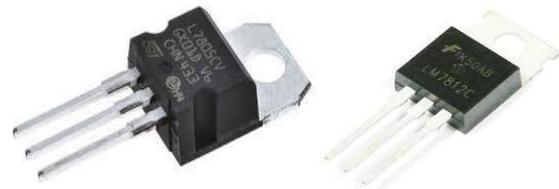
Fig. 7. Voltage Regulator 7805 and 7812
