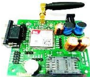
Fig. 5. Global system for mobile communication (GSM 800A)
