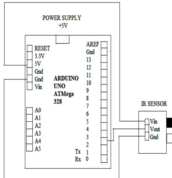
**Fig. 11.** IR Sensor and Arduino interfacing
