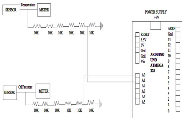
Fig. 4. Voltage Divider Connections
