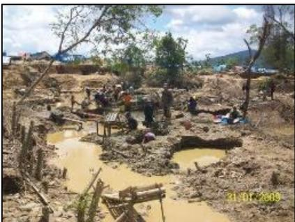
**Figure 3.** Typology: Excavation Technique (Well / Ditch)
