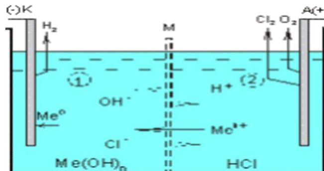
**Fig.1.** Electrolytic bath circuit for electrochemical activation of water
