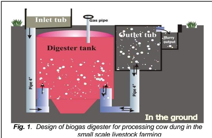
**Fig. 1.** Design of biogas digester for processing cow dung in the small scale livestock farming
