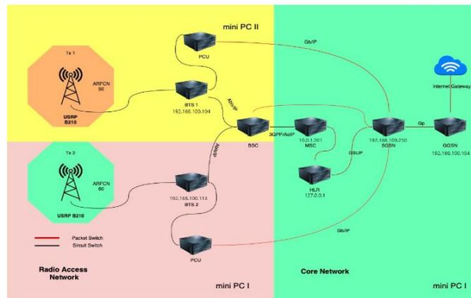
**Fig. 1. Proposed multi-site GPRS network architecture**
