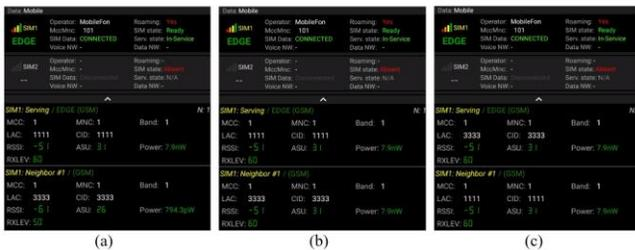
Fig. 11. Handover stages (a) initial serving cell, (b) Mobile Station approaching neighbour cell, (c) HO has succeeded.
