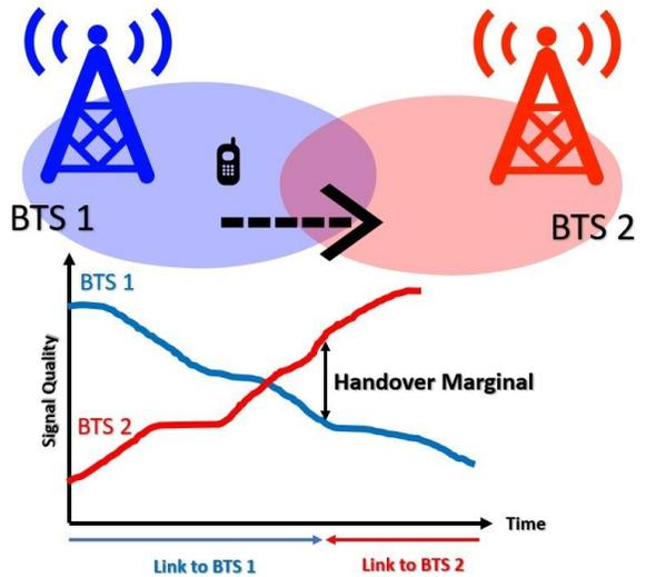
Fig. 6. The Handover mechanism based on power signal quality
