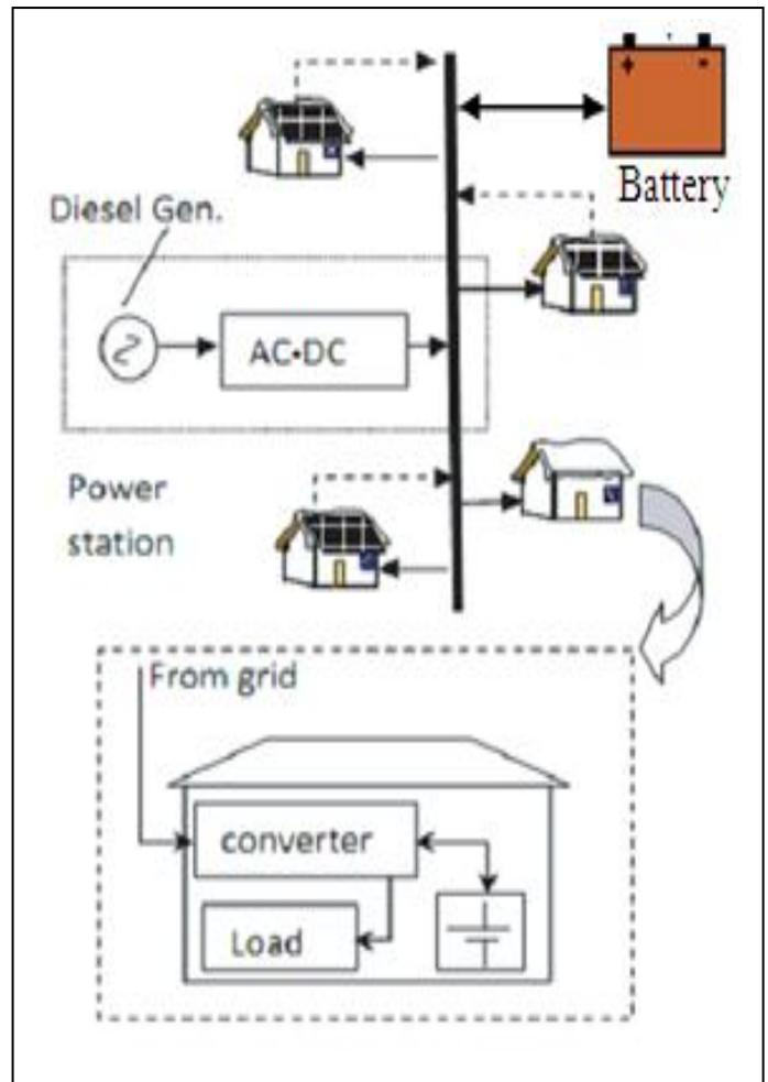
Fig. 3. The schematic diagram for the dc micro-grid. Dotted arrow marks show the connection from the PV panels to the grid.
