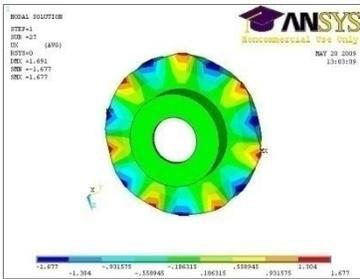
7th diametral disc mode shape plotted at frequency 11474.8 Hz
