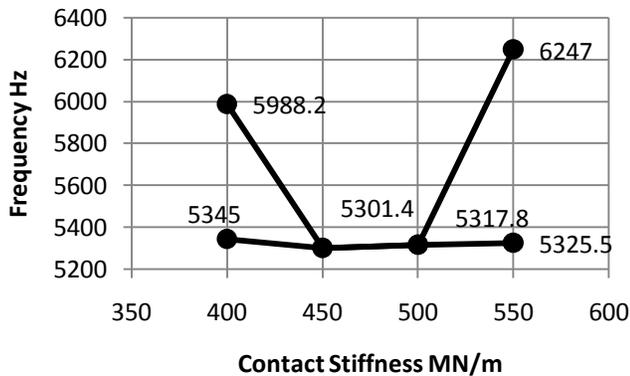
**Fig. 14. Effect of contact stiffness on the system mode frequencies at  $\mu=0.4$  for the system fourth mode shape**
