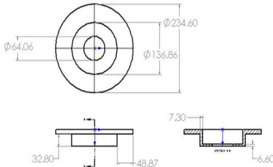
Fig. 2. Illustrates disc brake dimensions (all the dimensions in mm)
