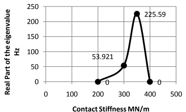
**Fig. 13. Effect of contact stiffness on the system instability at  $\mu=0.4$  for the system second mode shape.**
