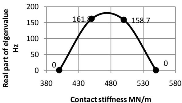
**Fig. 15. Effect of contact stiffness on the system instability at  $\mu=0.4$  for the system fourth mode shape**
