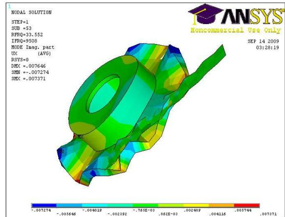
Fig. B. Mode shape at frequency 9507.7 Hz with contact stiffness 300 MN/m
