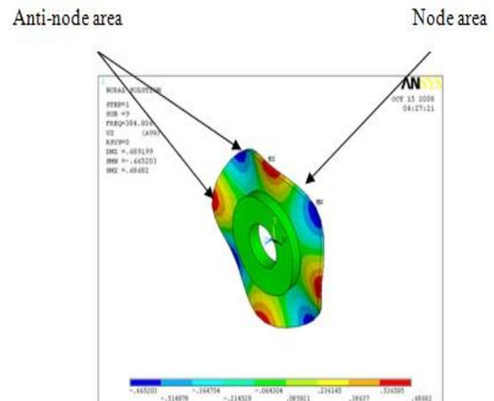
**Fig. 1. Illustrates the node and anti-node positions. The maximum amplitudes are referred to as antinodes and the apparent zero position as nodes**
