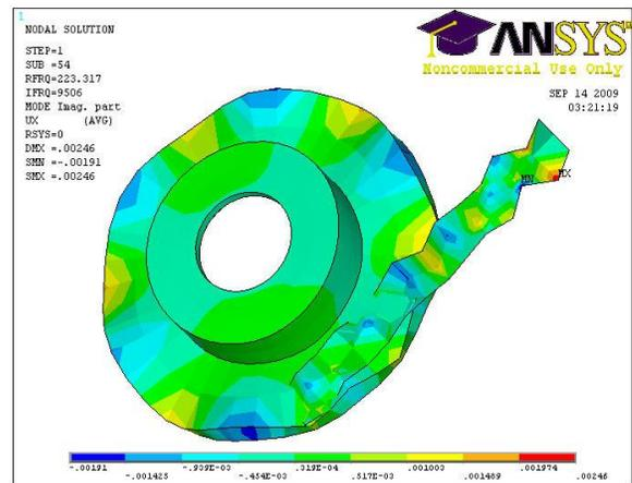
Fig. C. Mode shape at frequency 8809.8Hz with contact stiffness 350 MN/m
