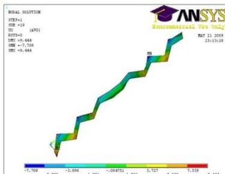
19th mode shape (bending),  $f=5235.3$  Hz
