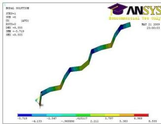
6th mode shape (bending),  $f=2236.7$  Hz
