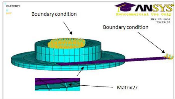
Fig. 8. Plate-Disc system coupled with matrix 27 as a contact element (Finite element model of Disc-plate system geometry)
