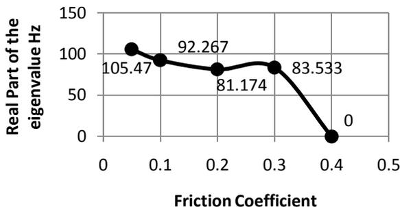
**Fig. 21. The effect of friction coefficient on the system instability at K=370 MN/m for the system second mode shape**
