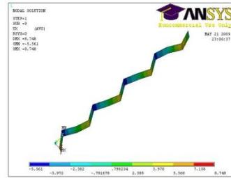
9th mode shape (bending),  $f=2878.4$  Hz
