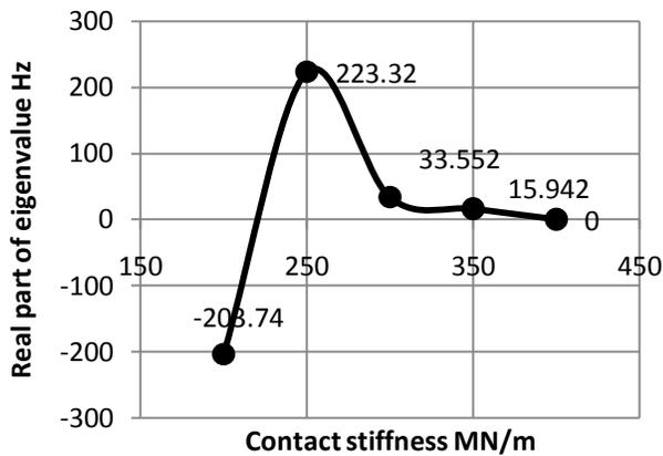
**Fig. 11. Effect of contact stiffness on the system instability at  $\mu=0.4$  for the system fifth mode shape**
