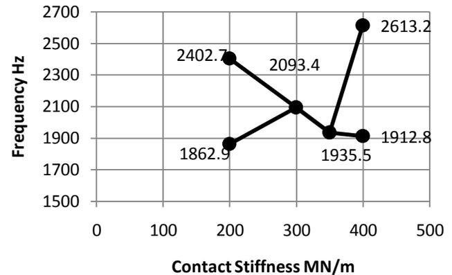
**Fig. 12. Effect of contact stiffness on the system mode frequencies at  $\mu=0.4$  for the system second mode shape.**
