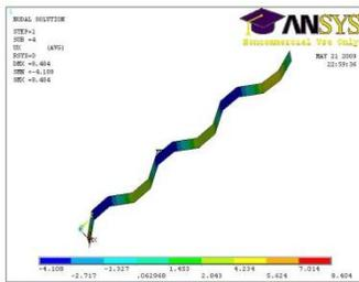
4th mode shape (bending),  $f=1675.1$  Hz
