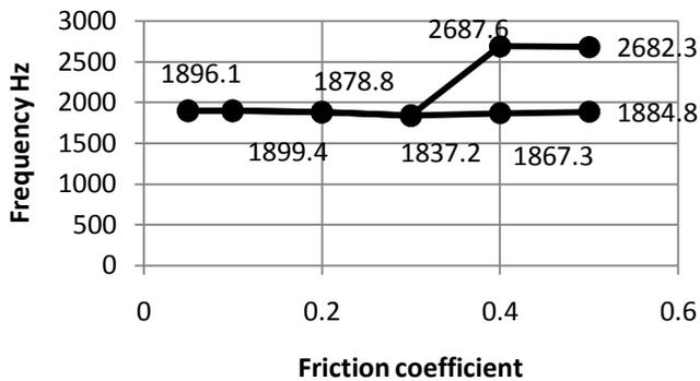
**Fig. 20. Effect of friction coefficient on the system mode frequencies at K=370 MN/m for the system second mode shape**
