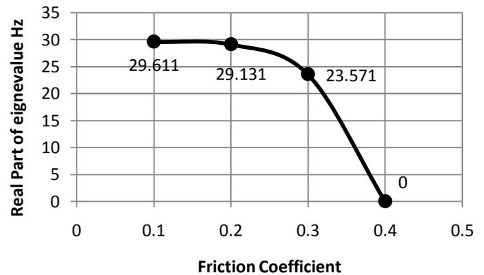
**Fig. 19. Effect of friction coefficient on the system instability at K=370 MN/m for the system third mode shape**
