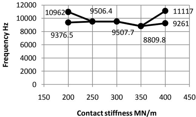
Fig. 9. Effect of contact stiffness on the system mode frequencies at  $\mu=0.4$  for the system sixth mode shape
