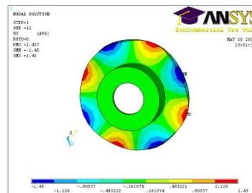
4th diametral disc mode shape plotted at frequency 4312.3 Hz
