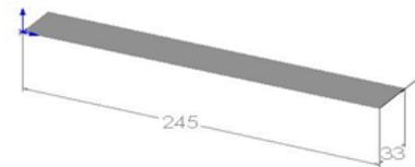
Fig. 5. Plate geometric dimensions, the entire dimension in millimeter
