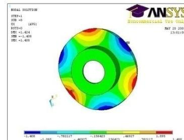
3rd diametral disc mode shape plotted at frequency 2944.6 Hz
