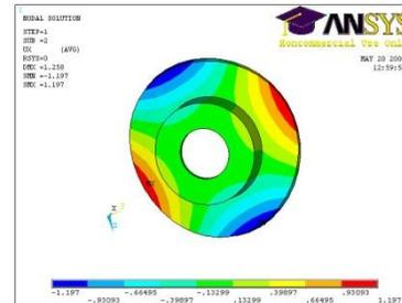
2nd diametral disc mode shape plotted at frequency 1808.2 Hz
