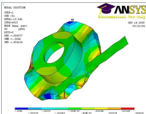
Fig. A. Mode shape at frequency 10692 Hz with contact stiffness 200 MN/m
