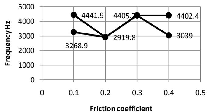
**Fig. 16. Effects of friction coefficient on the system mode frequencies at  $K=200$  MN/m for the system third mode shape**
