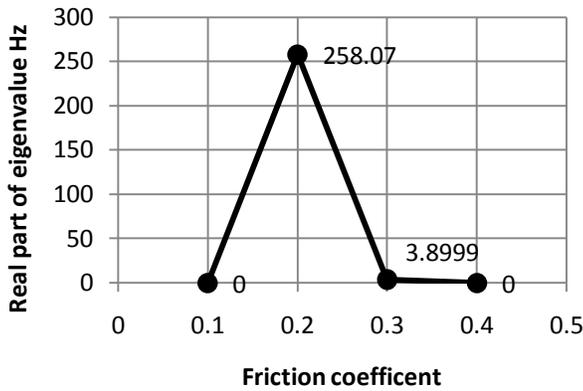
**Fig. 17. The effect of friction coefficient on the system instability at K=200 MN/m for the system third diametral mode shape**
