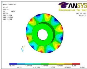
6th diametral disc mode shape plotted at frequency 8571.8 Hz
