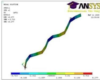
2nd mode shape (bending),  $f=1194.2$  Hz
