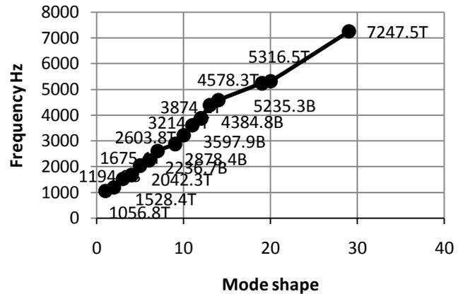
Fig. 7. Mode shape versus plate frequency, the B and T symbols refer to Torsion and Bending mode shape
