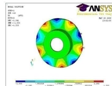
5th diametral disc mode shape plotted at frequency 6184.6 Hz
