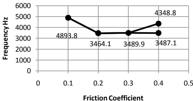
**Fig. 18. Effect of friction coefficient on the system mode frequencies at K=370 MN/m for the system third mode shape**
