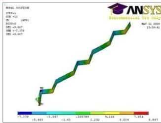
13th mode shape (bending),  $f=4384.8$  Hz
