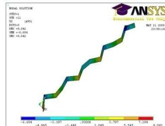
11th mode shape (bending),  $f=3597.9$  Hz
