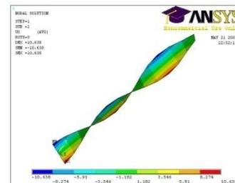
1st mode shape (torsion), f=1056.8 Hz
