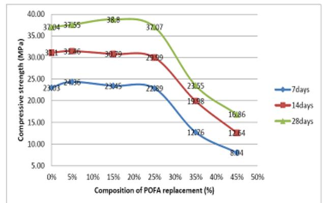
Figure 3: Average compressive strength verses curing days of concrete specimens
