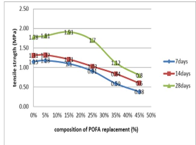
Figure 5: Tensile strengths variation with different percentages of POFA
