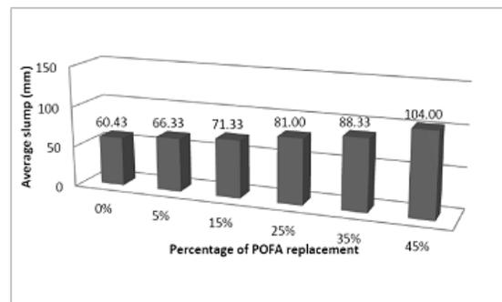
Figure 1: Results of Slump Test
