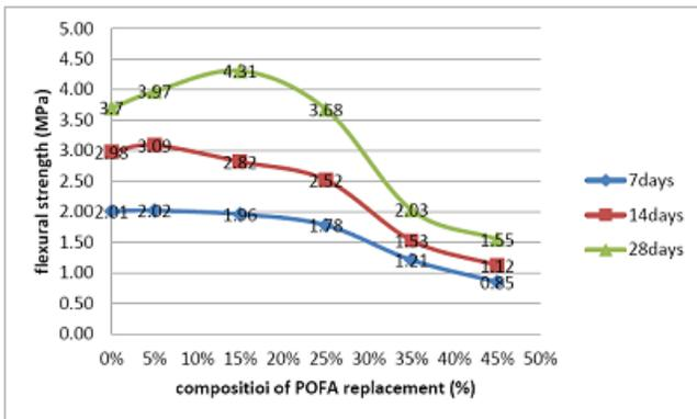
Figure 4: Average flexural strength versus curing days of concrete specimens
