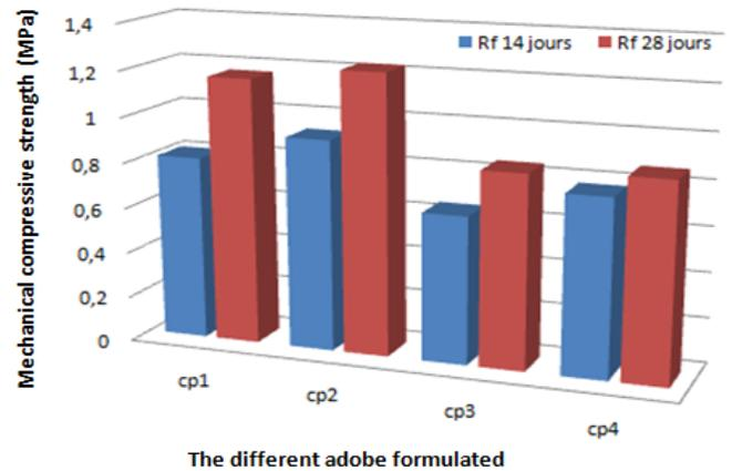
Fig.5. Mechanical compressive strength of adobe made
