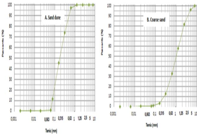
Fig. 4. Curve of particle size analysis of sands used. (a: sand dune b: coarse sand)
