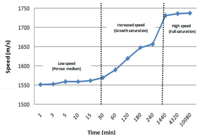
Fig.8. Changes in the speed of wave propagation as a function of moisture.
