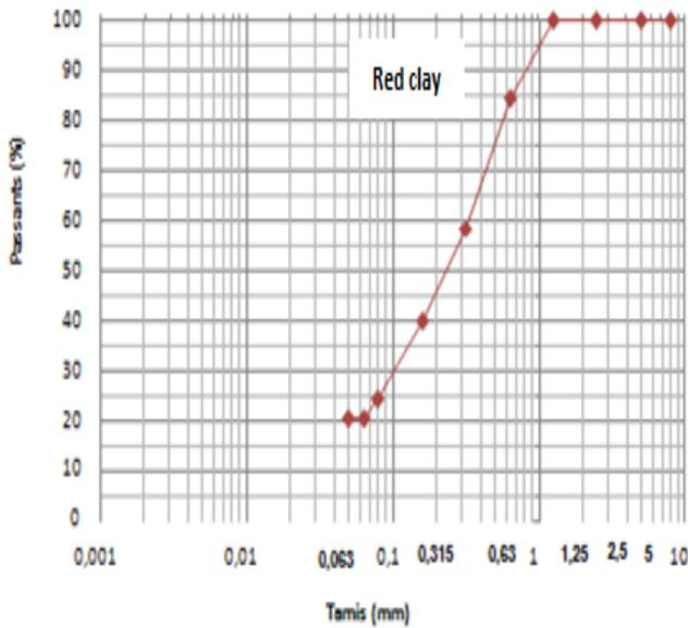
Fig.3. Curve of particle size analysis of the red clay.
