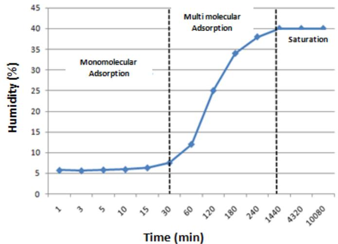
Fig. 7. Evolution of moisture as a function of time
