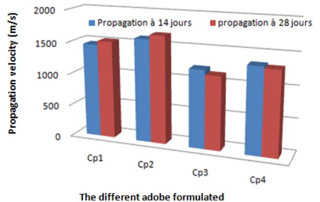
Fig.6. Histograms of time and speeds adobes made by the ultrasonic test.
