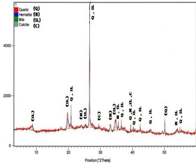
Fig .1. Mineralogical analysis of the red clay.
