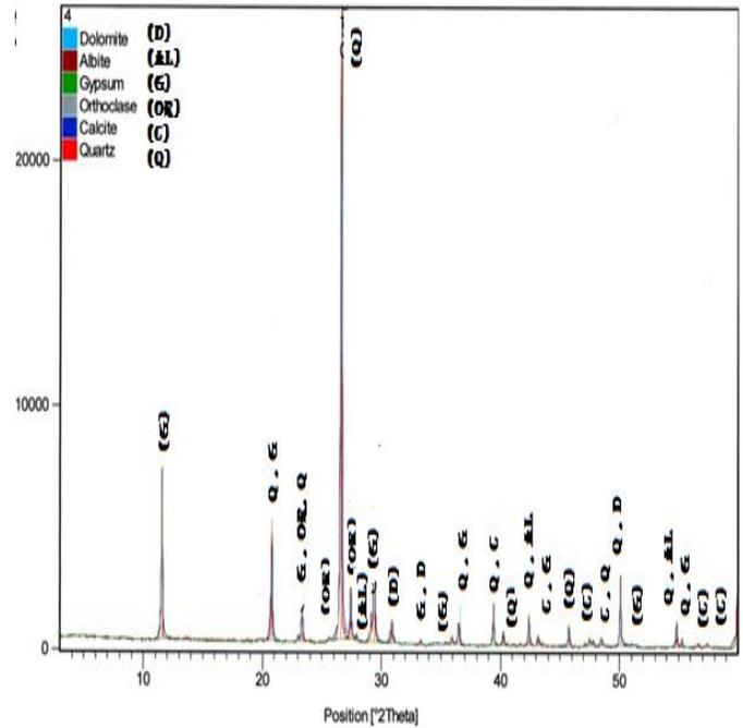
Fig .2. Mineralogical analysis of sand dune
