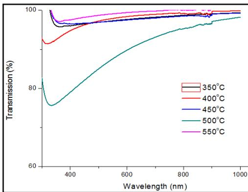
**Fig. 2** Transmittance spectra of as-deposited amorphous carbon films deposited at various temperatures for 1h with negative bias of -40V.
