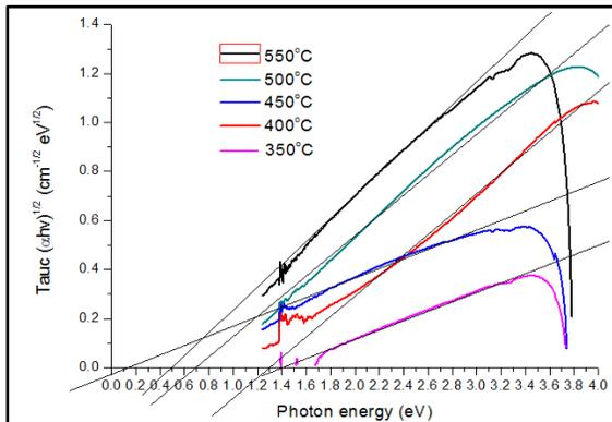
**Fig. 4** Optical band gap of as-deposited amorphous carbon films at various temperatures for 1h with negative bias of -40V.
