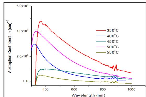
**Fig. 3** Absorption coefficient of non-doped amorphous carbon thin films deposited at various temperatures for 1h with negative bias of -40V.
