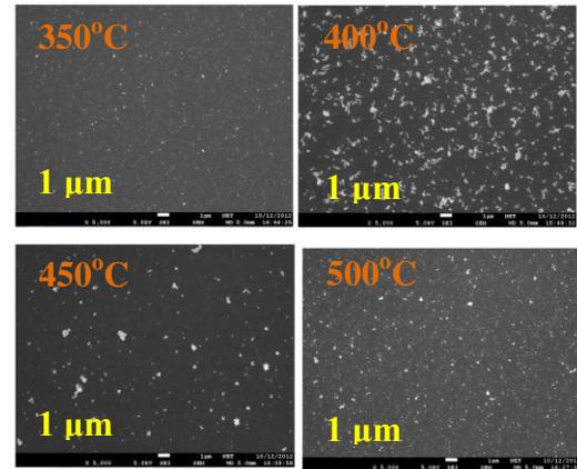
**Fig. 5** FESEM images for 1μm a-C thin film grown on p-type silicon at different temperatures: (a) 350°C, (b) 400°C, (c) 450°C, (d) 500°C by magnification 5k using 5.0kV
