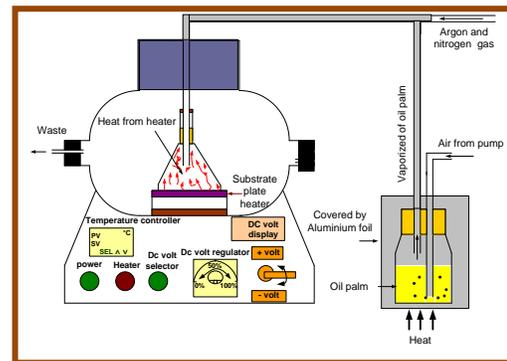
**Fig. 1.** A schematic diagram of bias assisted pyrolysis-CVD
