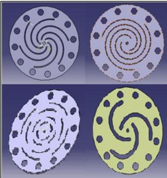
Fig 4.2 Catia model of different flexure
