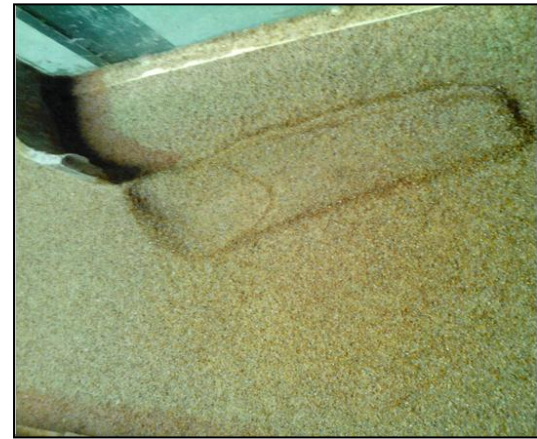
Fig. (3): Scour pattern at the end of a test
